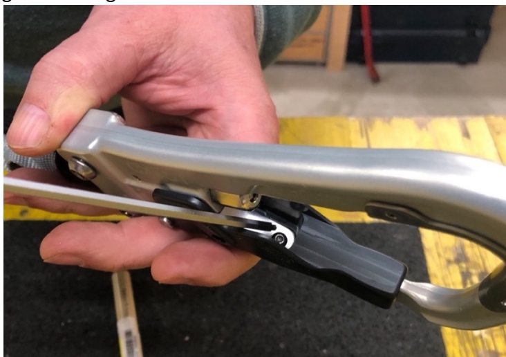
Figure 19: Fastening and gluing the screw
