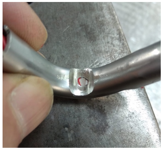
Figure 21: Worn abrasion guard - needs replacement
