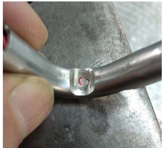
Figure 21: Worn abrasion guard - needs replacement
