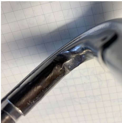
Figure 20:: Slightly worn abrasion guard - does not require replacement
