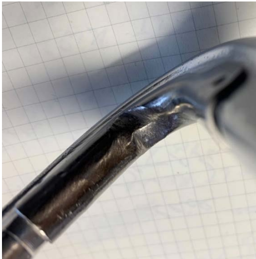
Figure 22:: Slightly worn abrasion guard - does not require replacement
