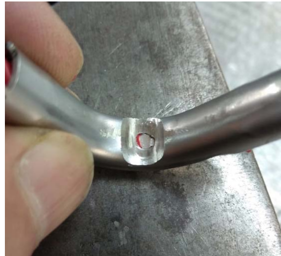
Figure 23: Worn abrasion guard - needs replacement
