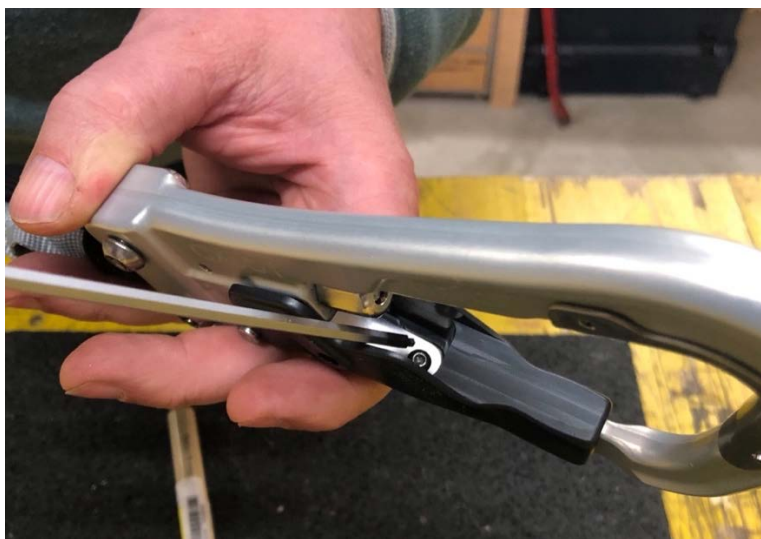
Figure 21: Fastening and gluing the screw
