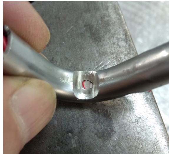
Figure 23: Worn abrasion guard - needs replacement
