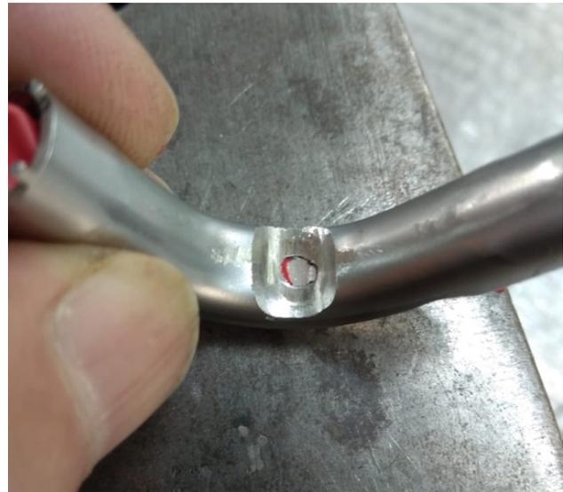
Figure 22: Worn abrasion guard - needs replacement
