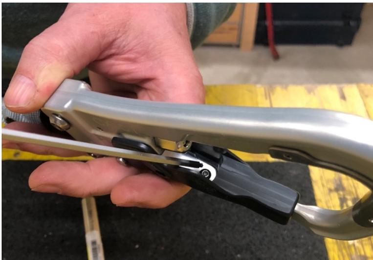
*Figure 20: Fastening and gluing the screw*
